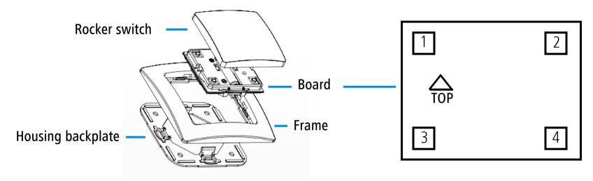
(3) If you fasten the Home Control Wall Switch using the double-sided tape for corners, put this tape on the four corners of the housing backplate and attach the Home Control Wall Switch to the place you want it to be.
